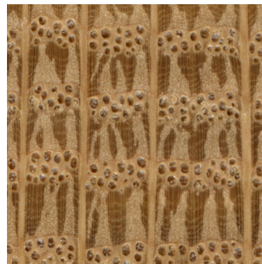
The pores in the heartwood of White Oak are plugged with tyloses, making them more difficult to see.
